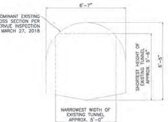
were carried out in 1981 and 1991 (Lachel & Associates 1991). In 2015, a multisensor robotic inspection was also performed (HDR Engineering 2016). This most recent condition assessment revealed that the tunnel needed rehabilitation and/or replacement due to deterioration of the shotcrete lining, ground water infiltration and other structural defects.
